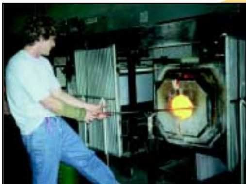
Figure 2. Glass artist Greg Fidler reheats a molten glass sample in the "glory hole" of a glass furnace.
